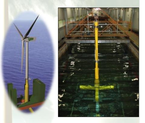
cases, but in other cases the numerical model failed to accurately predict the platform response. The results from both studies show the benefits of such TLP structures in terms of reduced motions which are vital to reliably obtain a high power output from a floating offshore wind turbine.
