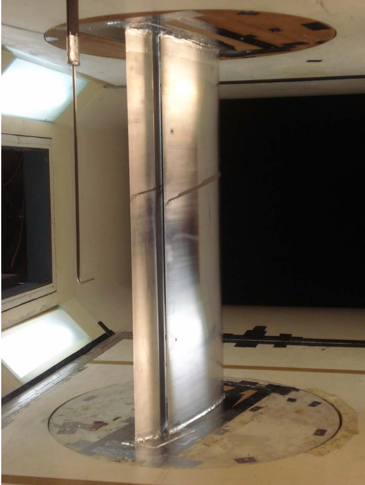
Figure 3.- S414 airfoil model and wake-survey probe mounted in test section.
