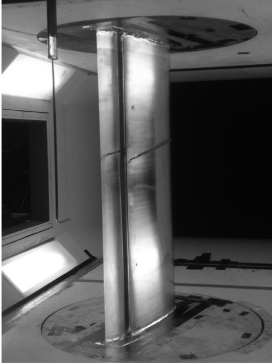
Fig. 4 S414 wind-tunnel model installed in the Pennsylvania State University Low-Speed, Low-Turbulence Wind Tunnel.
