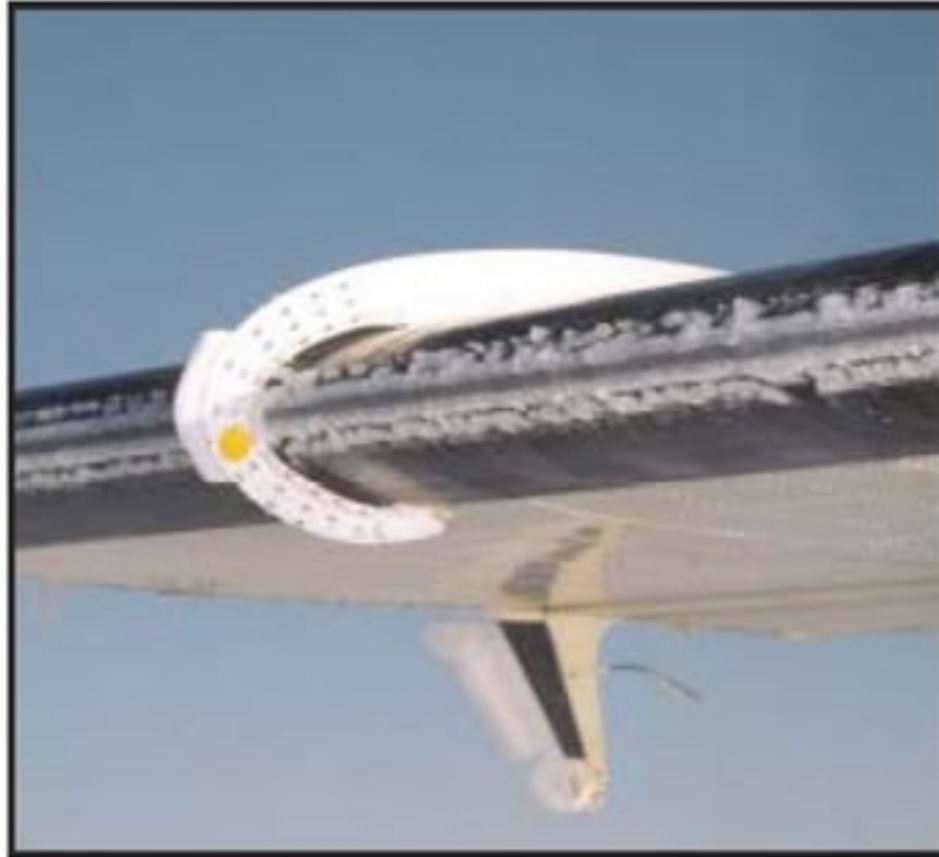
Mixed ice formation on wing leading edge
