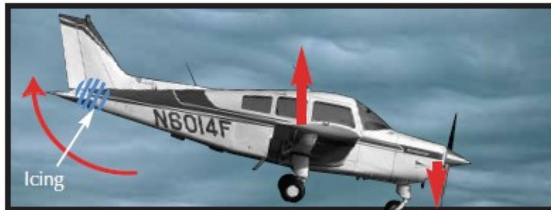
Tail stalls — loss of lift from horizontal tail
