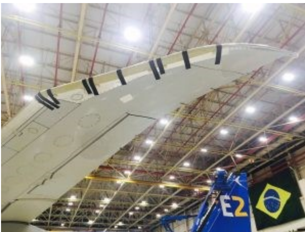
Flight testing with simulated ice shapes
