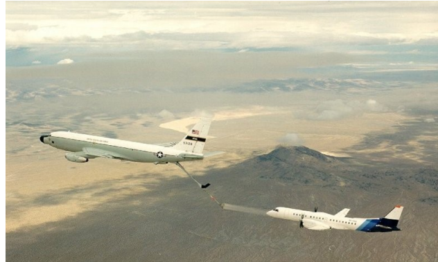
Flight testing in a simulated cloud produced by an icing tanker
