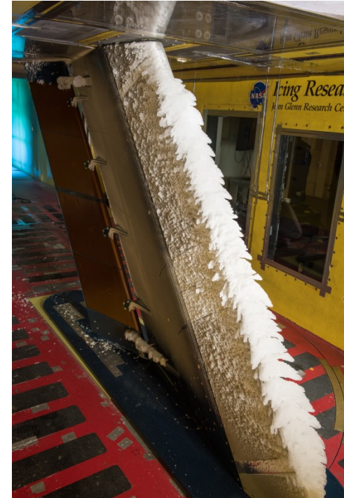
Ground testing in icing wind tunnels
