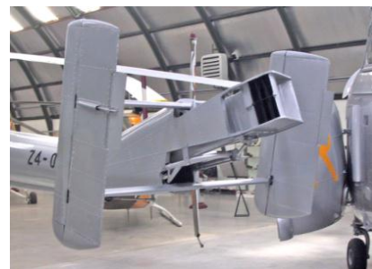
Figure 25. Aerotécnica AC-14 Directed Jet Thruster with Additional Forward Thrust Ability
