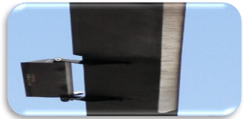
Figure 21. Servo flap on the Kaman K-Max
