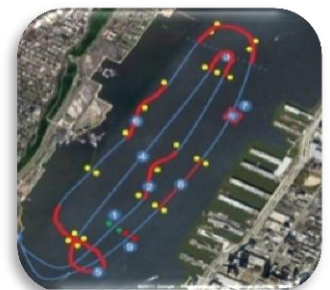
Figure 23. Highlighted portions indicate yawing maneuvers throughout the course
