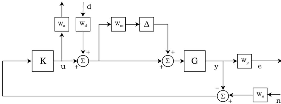
Figure 6: *Block Diagram of Robust Controller*
