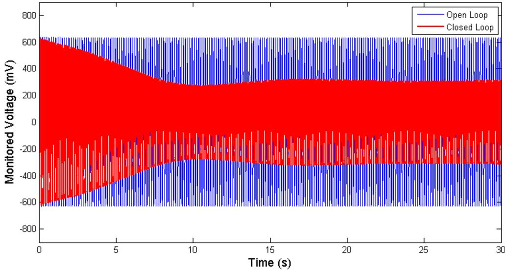
Figure 10: *Open and Closed Loop Time Responses of First Mode Forced Vibration (Monitored by Piezoelectric Patch 2A)*
