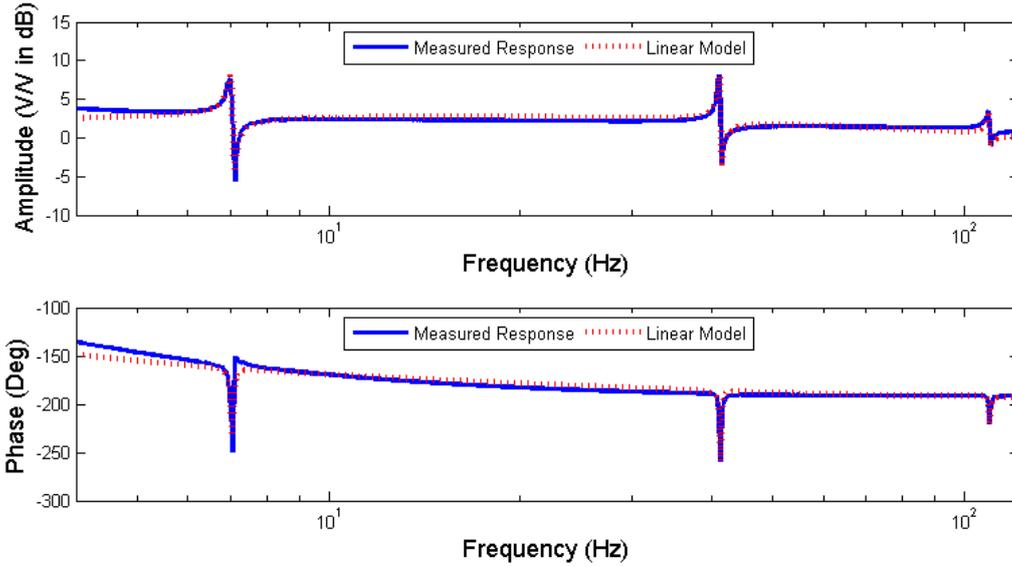
Figure 5: *Experimental Frequency Response and Linear Model for Smart Beam using Self-Sensing Piezoelectric Actuator*
