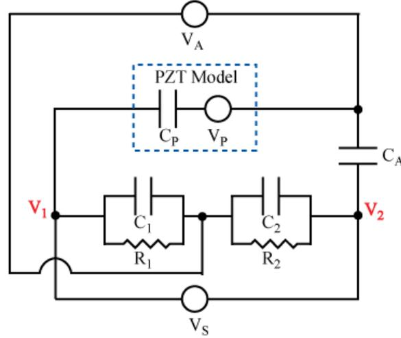
Figure 4: *Bridge Circuit for Self-Sensing Actuator*
