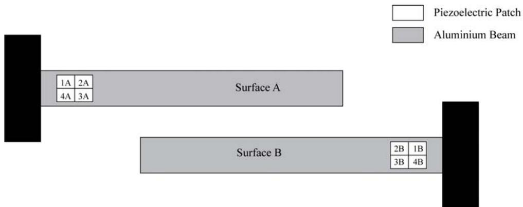
Figure 3: *Piezoelectric Patches on Smart Beam*
