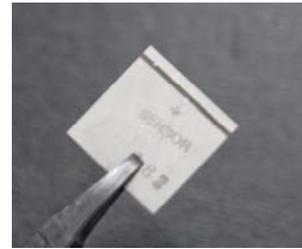
Figure 2: *SensorTech - BM500 PZT Patch*
