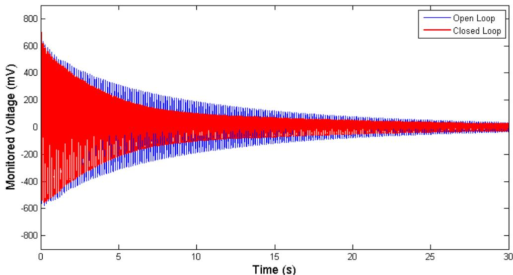
Figure 9: *Open and Closed Loop Time Responses of Free Vibration (Monitored by Piezoelectric Patch 2A)*
