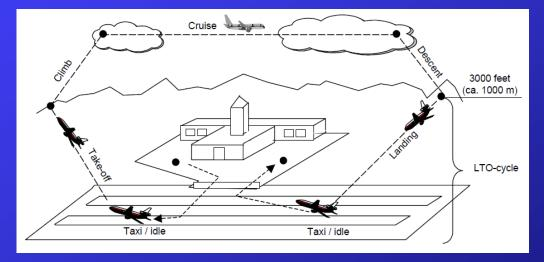
Landing and take-off cycle (LTO), which comprises all activities near the airport; and the cruise section, which is defined by all the activities taking place above 1000m. [1] and [2] estimate that 5-20% of the fuel consumed throughout the flight is due to the LTO cycle. Hence an optimum wing for LTO can provide lower emission. 9/14
