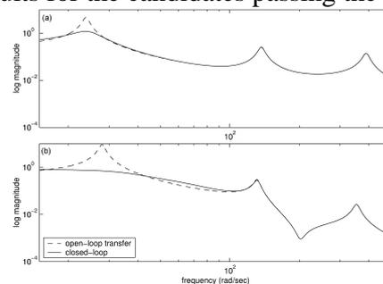
Figure 10. The comparison of the open and closed-loop responses (a: initial configuration, b: maximum attenuation ratio;  $x_1=9, x_2=250, s_1=150, s_2=50$ , in mm)
