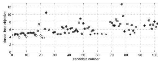
Figure 8. The comparison of the open-loop and closed-loop objective functions (o: candidates passing the feasibility test, \*: closed-loop objective)
