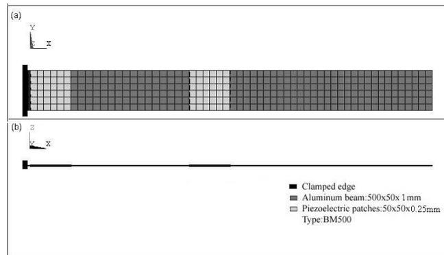
Figure 3. The finite element model and the initial size and configuration of the piezoelectric patches of the flexible structure ( a. Top view, b. Side view)
