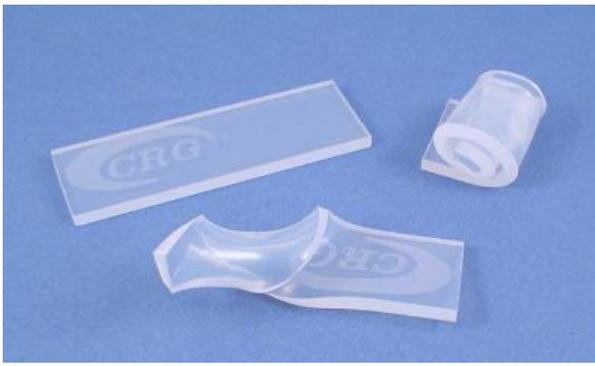
Fig. 11. A shape memory polymer used for morphing air vehicle applications [26].
