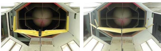
Fig. 4. Active winglet concept for drag reduction [4].
