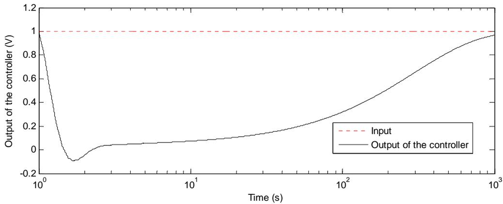
Fig. 11: Output voltage of the  $PI^\lambda D^\mu$  controller for step input
