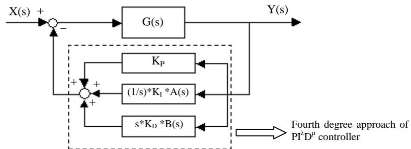
Fig. 3: Closed loop system
