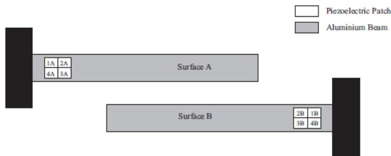
Fig. 2: Piezoelectric patches on smart beam
