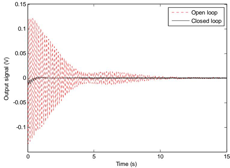
Fig. 6: Free vibration response of the smart beam
