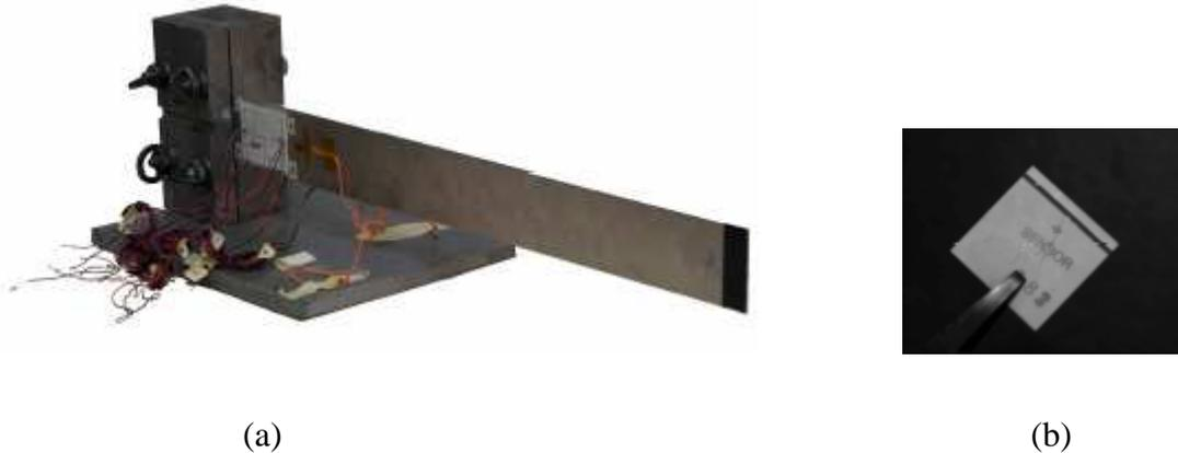
Fig. 1: (a) Smart beam (b) Piezoelectric patch (SensorTech - BM500 PZT Patch)
