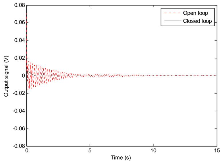
Fig. 7: The response of the smart beam to transient input
