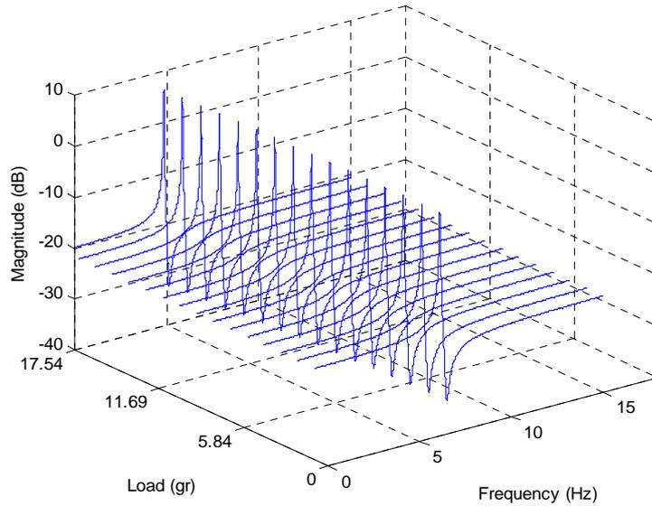
**Fig. 4:** Frequency responses of LPV modelled smart beam for various tip loads
