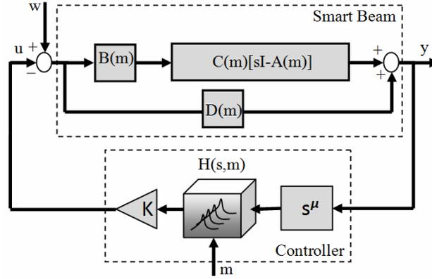
**Fig. 5:** LPV based fractional closed loop system
