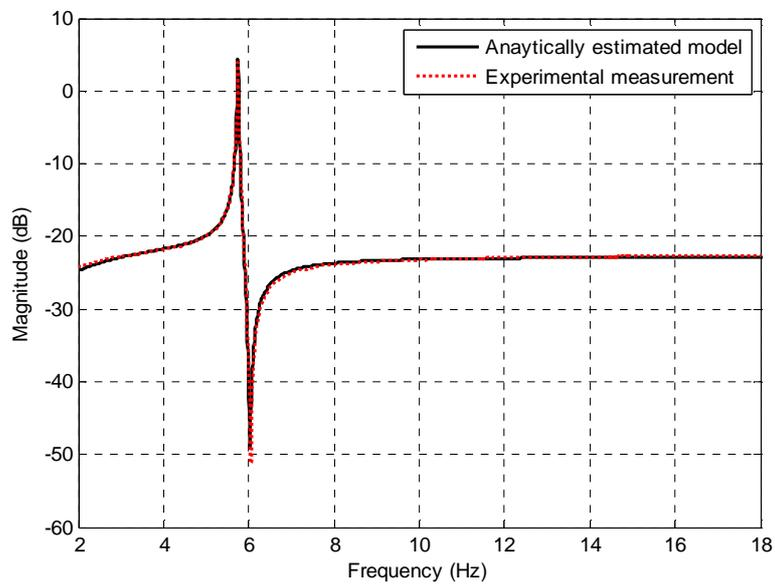
**Fig. 3:** Analytically estimated  $G_M(s)$  and experimentally measured transfer functions of the LPV modelled smart beam around its first mode (tip mass=17.54 [gr])
