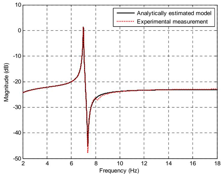
**Fig. 2:** Analytically estimated  $G(s)$  and experimentally measured transfer functions of the LPV modelled smart beam around its first mode
