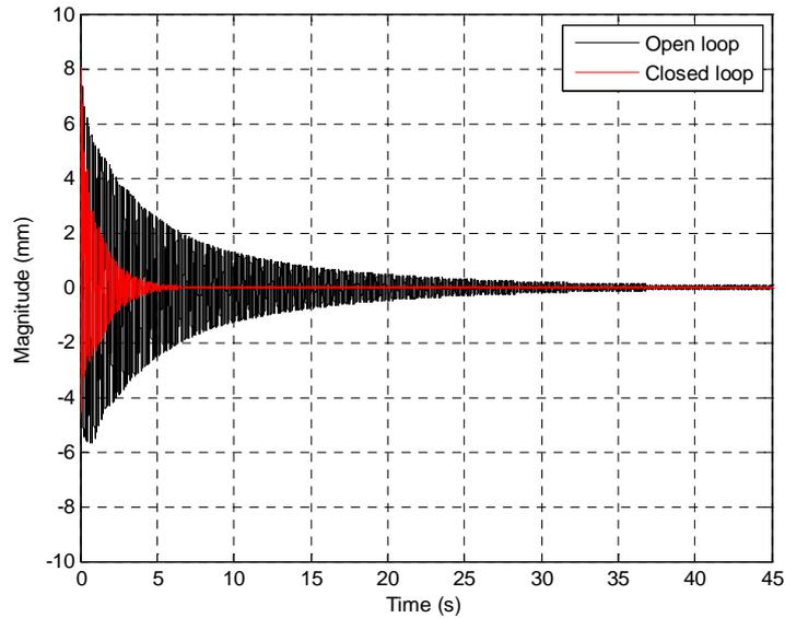
**Fig. 6:** Time domain response of free vibrations of the LPV modelled smart beam for unloaded case
