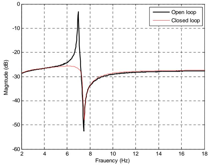
**Fig. 10:** Open and closed loop frequency responses of the LPV modelled smart beam for unloaded case
