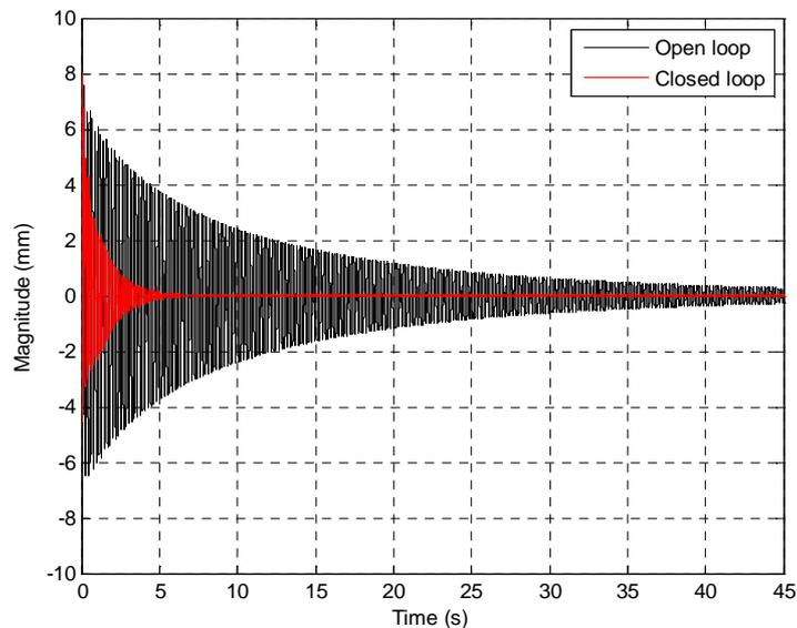
**Fig. 7:** Time domain response of free vibrations of the LPV modelled smart beam for fully loaded case (tip mass=17.54 [gr])
