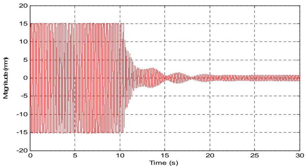
**Fig. 9:** Time domain response of free vibrations of the LPV modelled smart beam for fully loaded case (tip mass=17.54 [gr])
