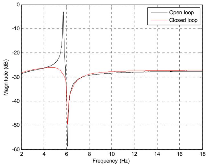
**Fig. 11:** Open and closed loop frequency responses of the LPV modelled smart beam for fully loaded case (tip mass=17.54 [gr])
