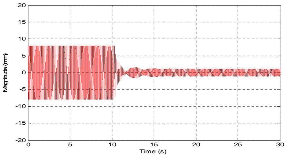
**Fig. 8:** Time domain response of forced vibrations of the LPV modelled smart beam for unloaded case
