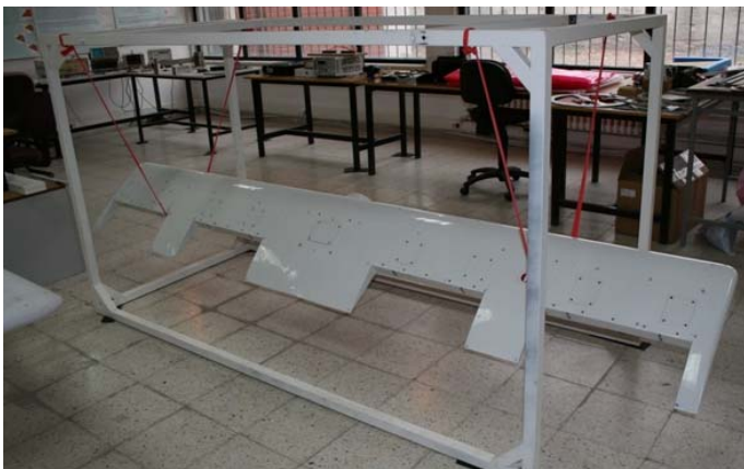
Figure 10 - Simulated Free-free Boundary Conditions in Laboratory
