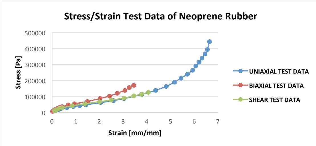
**Figure 5.** Stress/Strain Test Data of Neoprene Rubber
