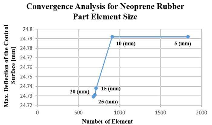
Figure 7. Convergence Analyses - for Composite Part (Left) and for Neoprene Rubber Part (Right)
