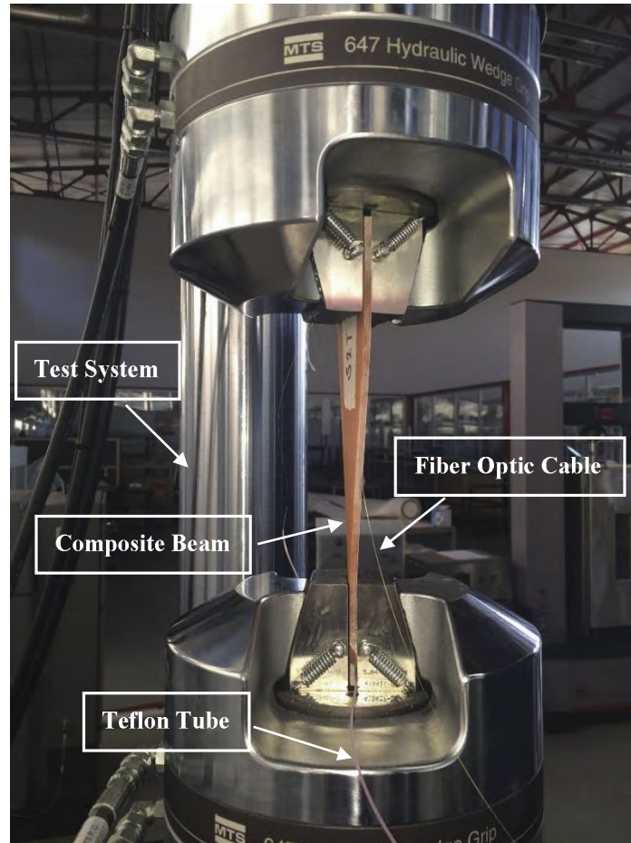
Figure 7. Composite Beam with Embedded FBG Sensors Mounted to the MTS 809 Axial/Torsional Test System
